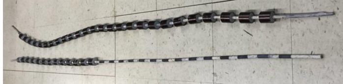
Fig. 1 Two riser models with buoyancy modules of 100% (top) and 50% (bottom) coverage ratio (length of the riser section with buoyancy modules to the total riser length). Black and white paint is used as the marker for motion tracking in the experiment.
