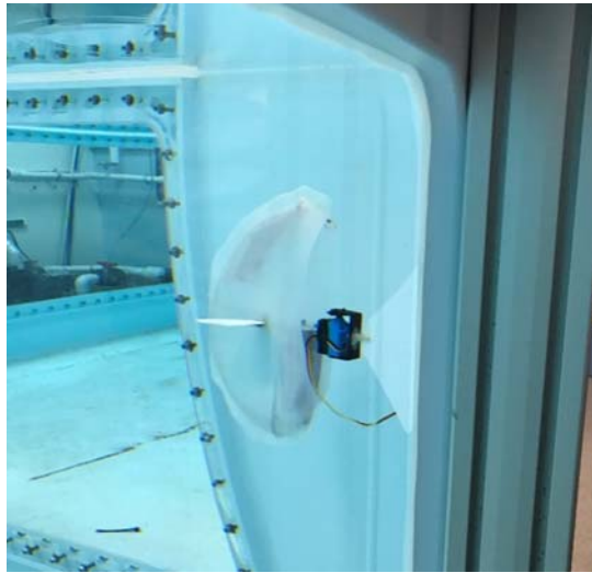
Fig. 6. Angel Fish-Inspired Robot in testing tank. Body to the left, tailfin to the right, blue RC servo in the middle. Approximately 41cm long and 30cm from dorsal to ventral.
