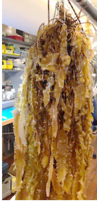
Figure 2. The 40 in-wide kelp bundle tested on July 17th, 2020. The kelp fronds, including the stipe and the blade, have a maximum length of 1.8 m.
